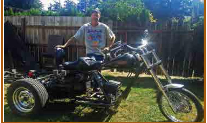
Jeff White, OR This is going to be a 2015 mid-engine Corvair trike. 3 degree rake front end, 140 hp wish me -luck
