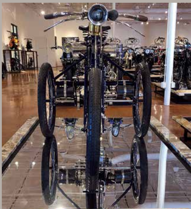
Peugeot Tricycle 2-1/4 HP 1899 Powered by the famous De Dion Bouton single cylinder engine, this late 19th century Peugeot was painstakingly restored in Holland by Gilbert Warming. This testament to the pioneer days of motorcycling is exceedingly rare and genuine, retaining many of the original components, notably including its De Dion engine and Peugeot two-speed gearbox.
